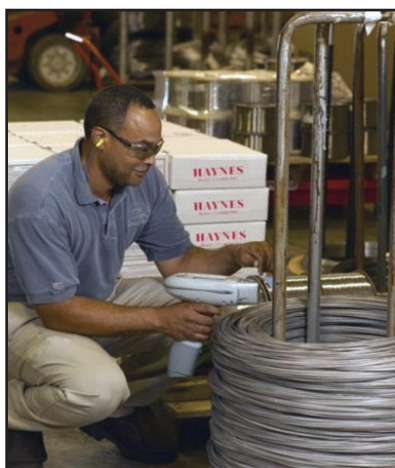
Rigorous positive material identification checks are built into every product.
